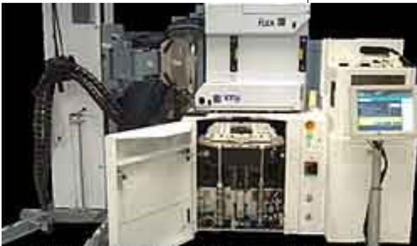
**Teradyne Ultra Probe Test Cell**
